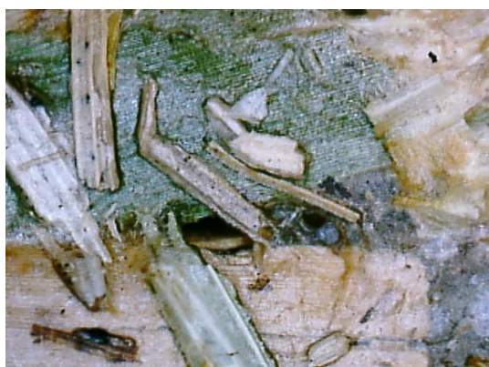
Fig. 5. Fine particles of reeds and rushes on the background of large pieces. Optical microphotography, magnification 20x
