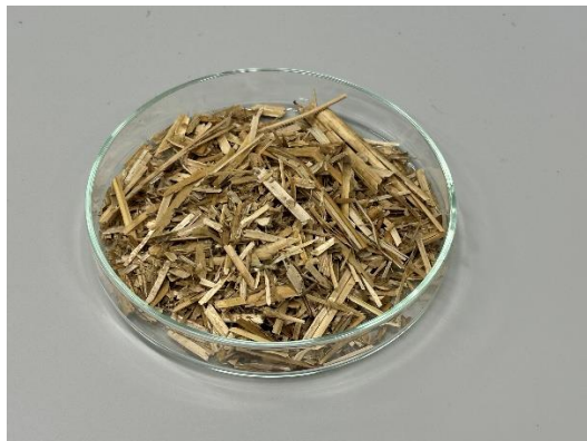
Fig. 1. Sample of crushed common reed ( Phragmites australis ). 3-4 cm long fibres dominate, with powdery filling
