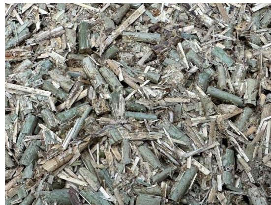
Fig. 4. Close-up view. Reed fibres arranged in random directions between pieces of bulrushes
